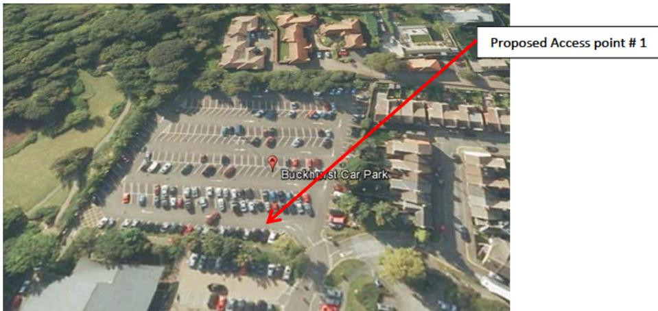
We envisage the deck should be located adjacent to the three unoccupied boundaries of the site Fig.1, leaving the boundary adjacent to the residential properties 20m clear of the proposed car deck to the rear of the residential structure.
